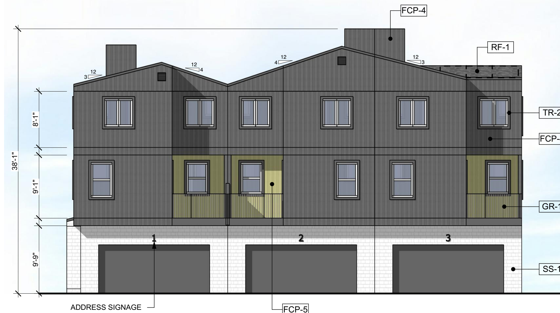
BUILDING 3 - SOUTH ELEVATION SCALE: 1/8" = 1'-0"
