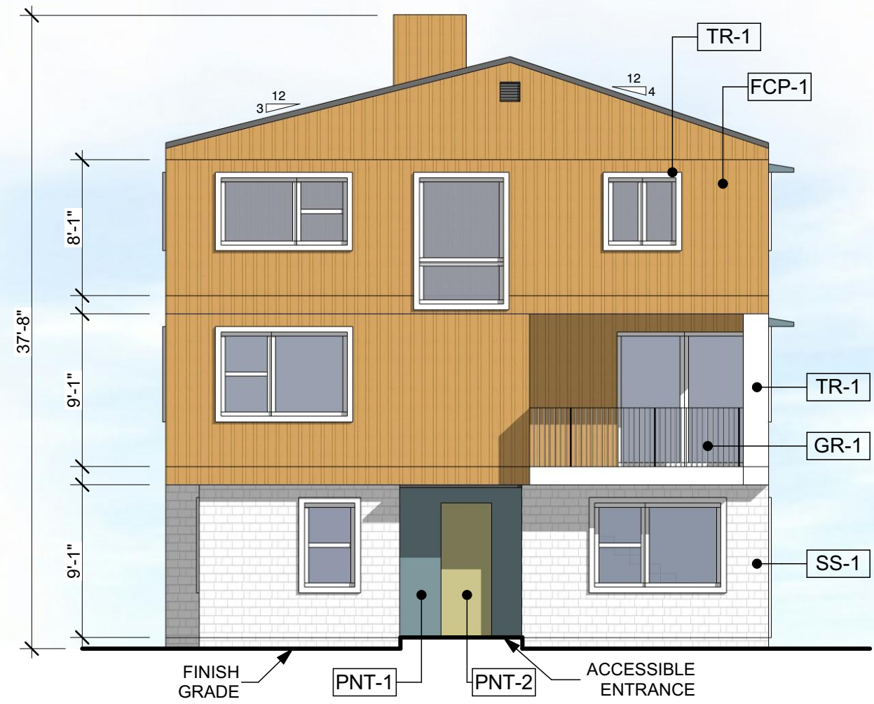
BUILDING 1 - WEST ELEVATION SCALE: 1/8" = 1'-0"
