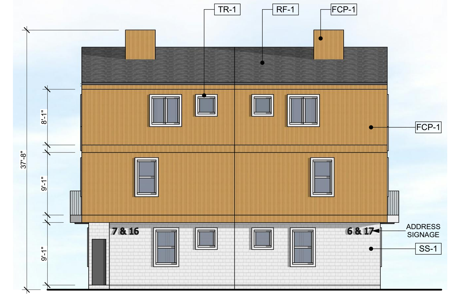
BUILDING 1 - NORTH ELEVATION SCALE: 1/8" = 1'-0"
