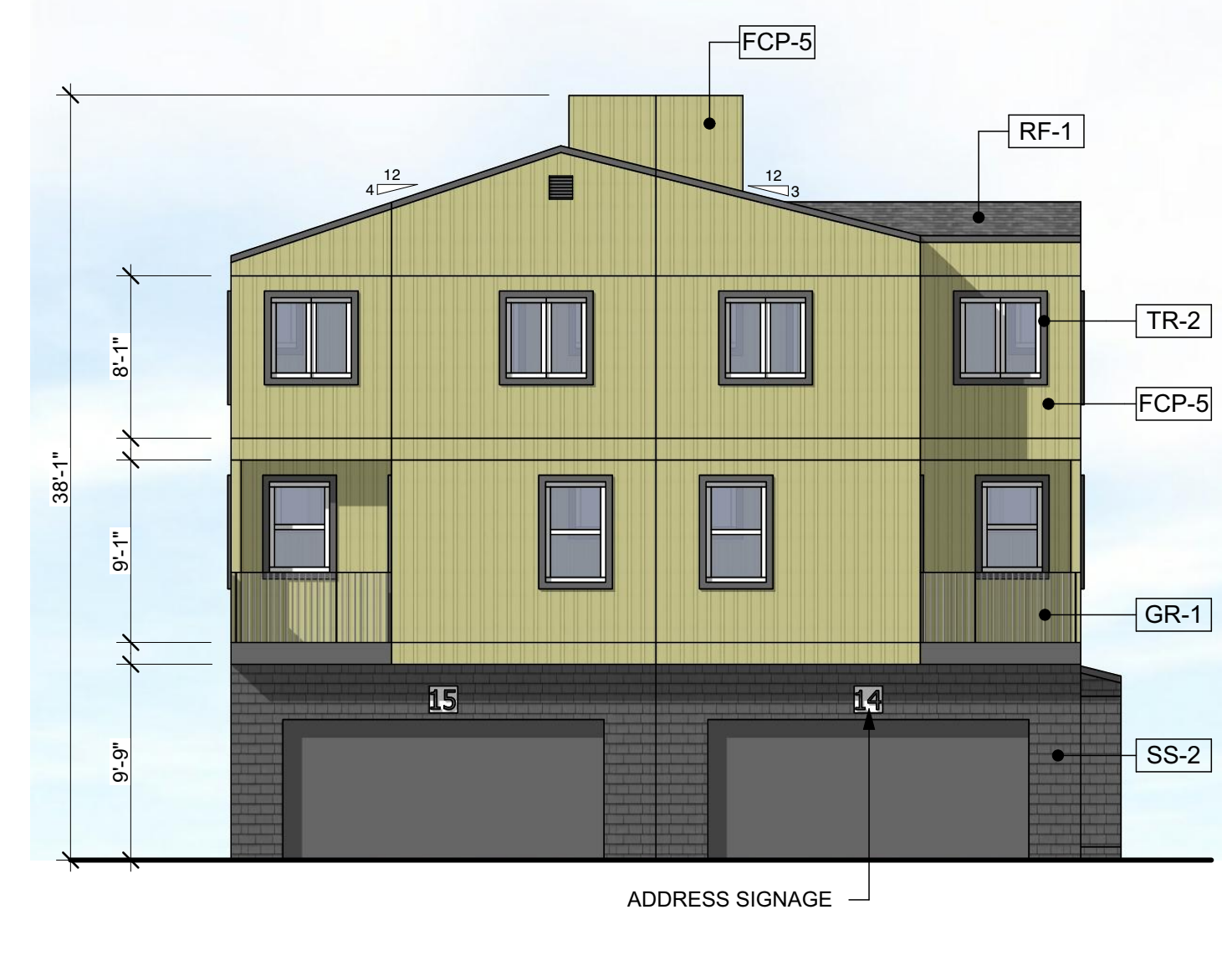
BUILDING 4 - NORTH ELEVATION SCALE: 1/8" = 1'-0"
