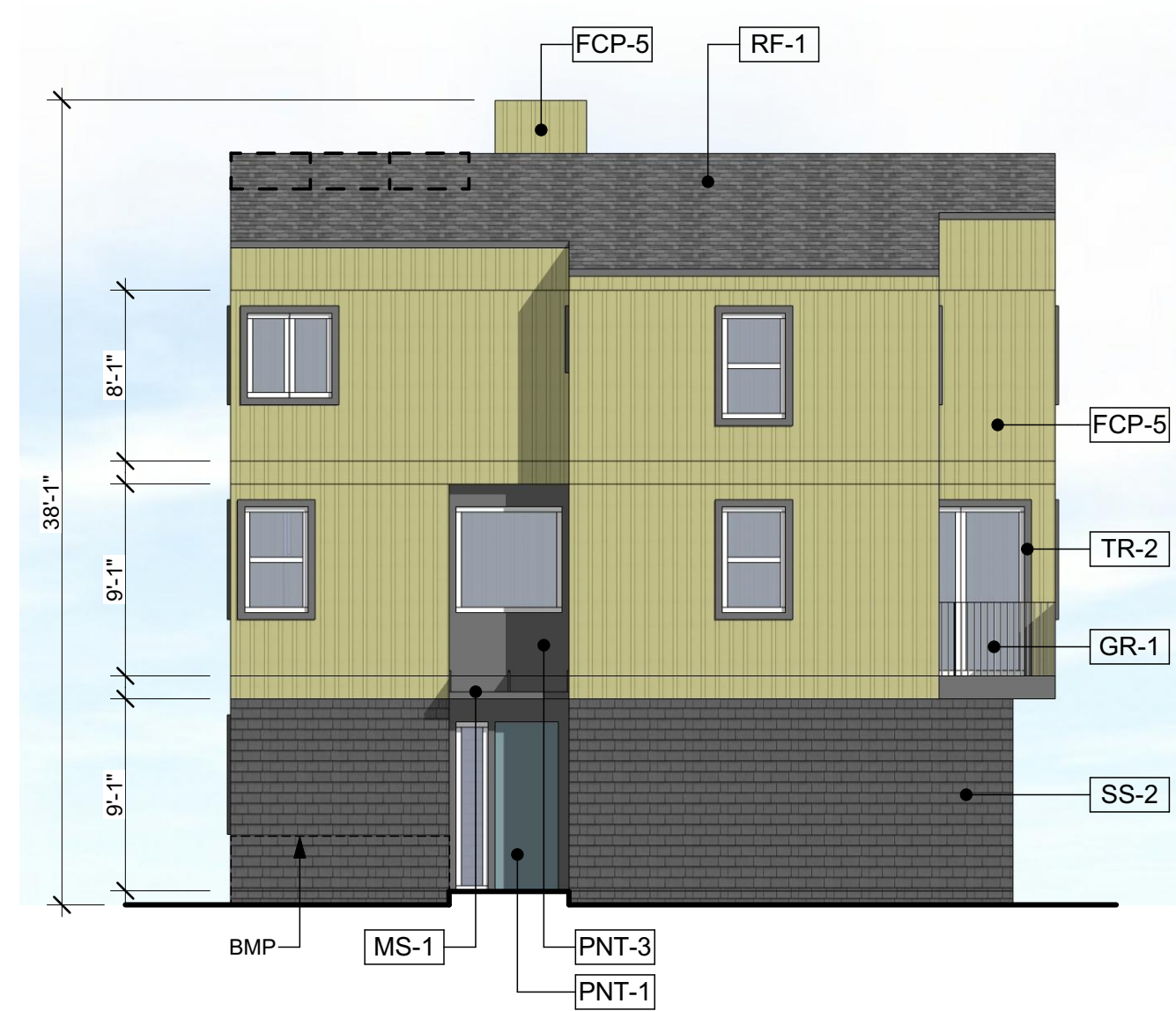
BUILDING 4 - EAST ELEVATION SCALE: 1/8" = 1'-0"
