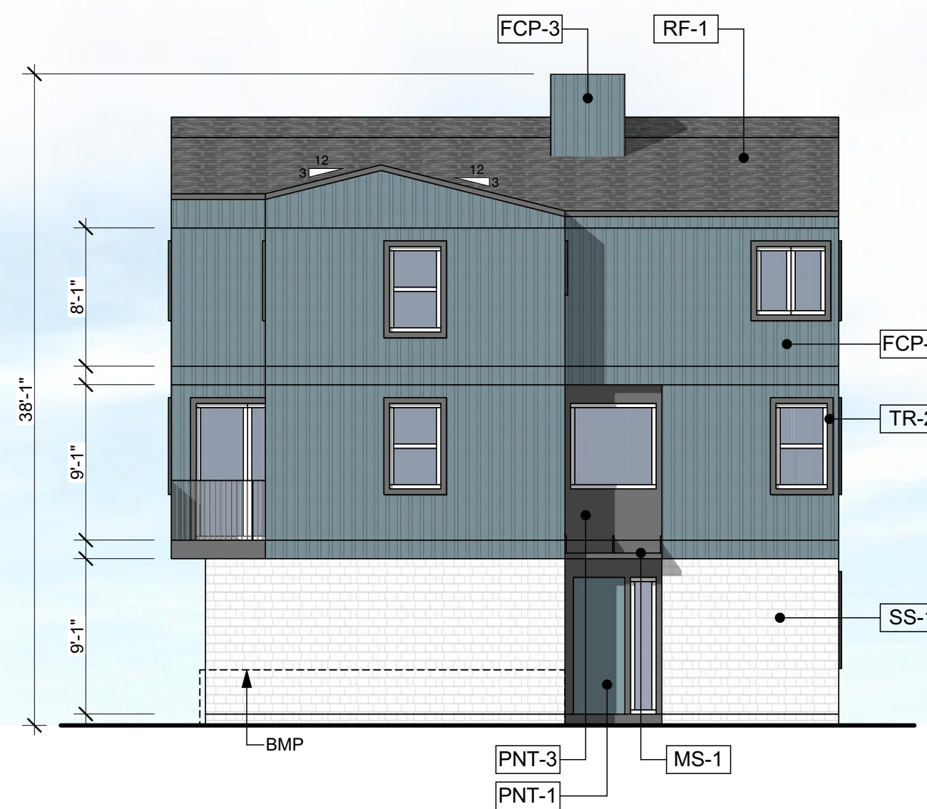
BUILDING 5 - EAST ELEVATION SCALE: 1/8" = 1'-0"
