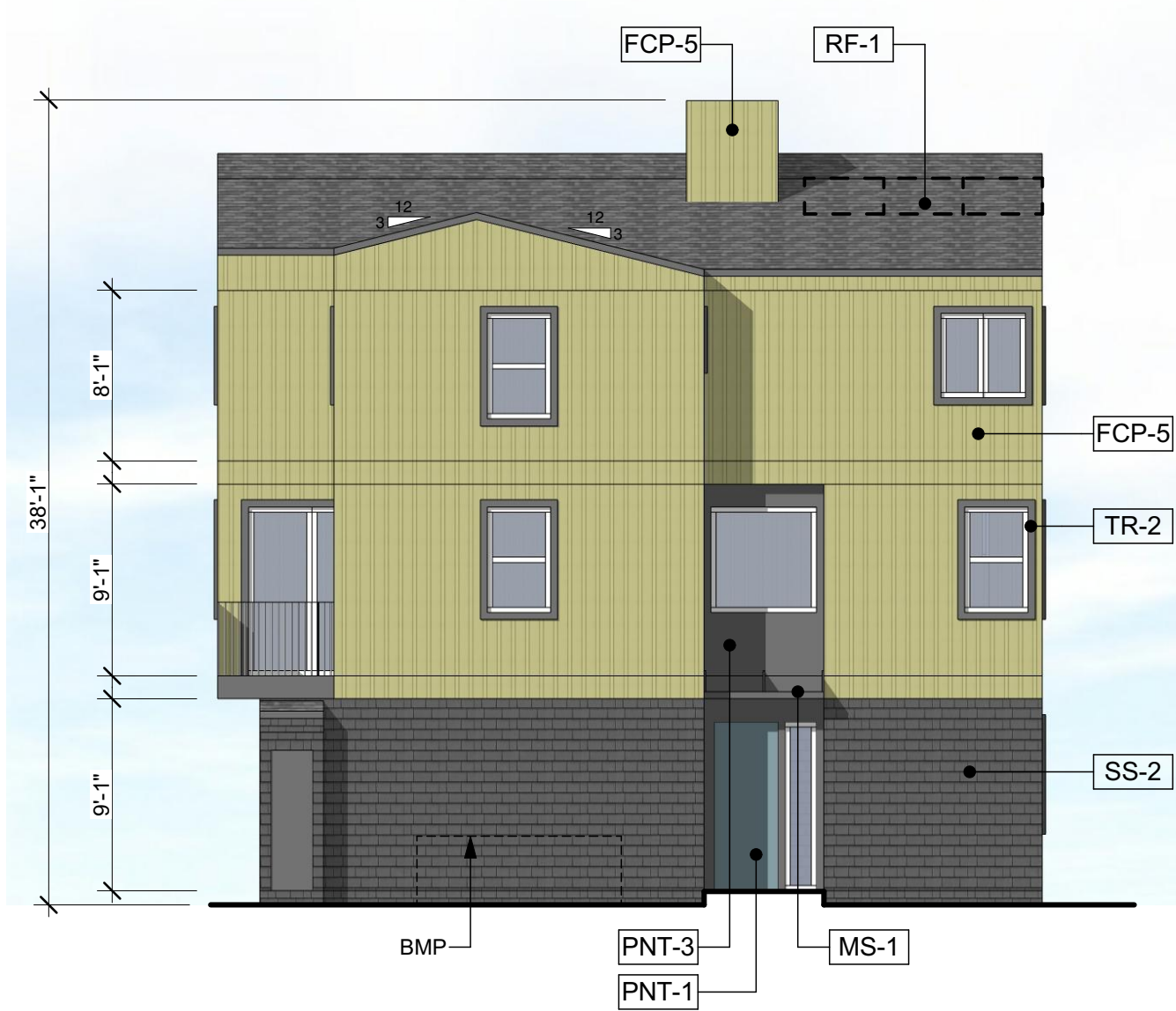
BUILDING 4 - WEST ELEVATION SCALE: 1/8" = 1'-0"
